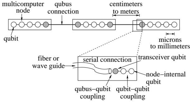
Figure 1: Quantum portions of our quantum multicomputer
