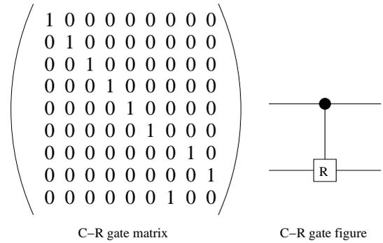
Figure 2: The control-rotor gate.
