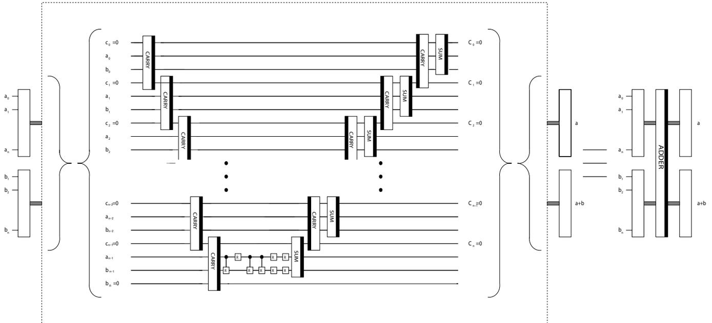
Figure 5: The complete ternary carry-ripple adder.
