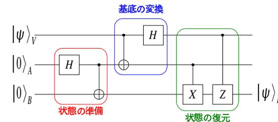
$$|\psi\rangle|0\rangle \xrightarrow{H_A} |\psi\rangle \otimes \frac{1}{\sqrt{2}}(|0\rangle + |1\rangle) \otimes |0\rangle \xrightarrow{C_{AB}} |\psi\rangle \otimes \frac{1}{\sqrt{2}}(|00\rangle + |11\rangle)$$
