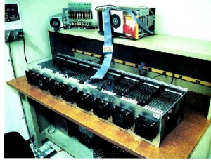
Caltech Cosmic Cube, 64 processors (8086/7) 3MFLOPS, 8MB RAM, 1982 (prototype)
