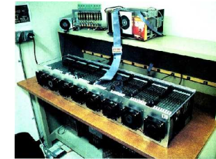
Caltech Cosmic Cube, 64 processors (8086/7) 3MFLOPS, 8MB RAM, 1982 (prototype)
